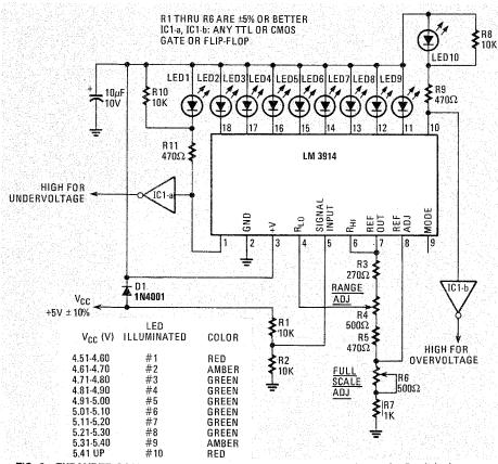
FIG. 2—EXPANDED-SCALE VOLTMETER for monitoring the output voltage of a 5-volt logic-power supply. Each LED corresponds to a predetermined voltage, as shown in the chart.
