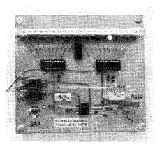
mic voltage-divider for a 3-dB-per-step display; otherwise, it's identical to the LM3914. The LM3915 is useful for displaying signals with wide dynamic range, such as RF signal strength, power level, or light intensity, in addition to audio level.
