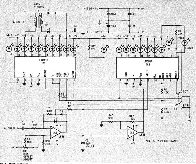
FIG. 5—TWO LM3915's can be cascaded together to obtain wide dynamic range. The circuit shown above is a peak-reading audio-level meter with a dynamic range of 60 dB.
